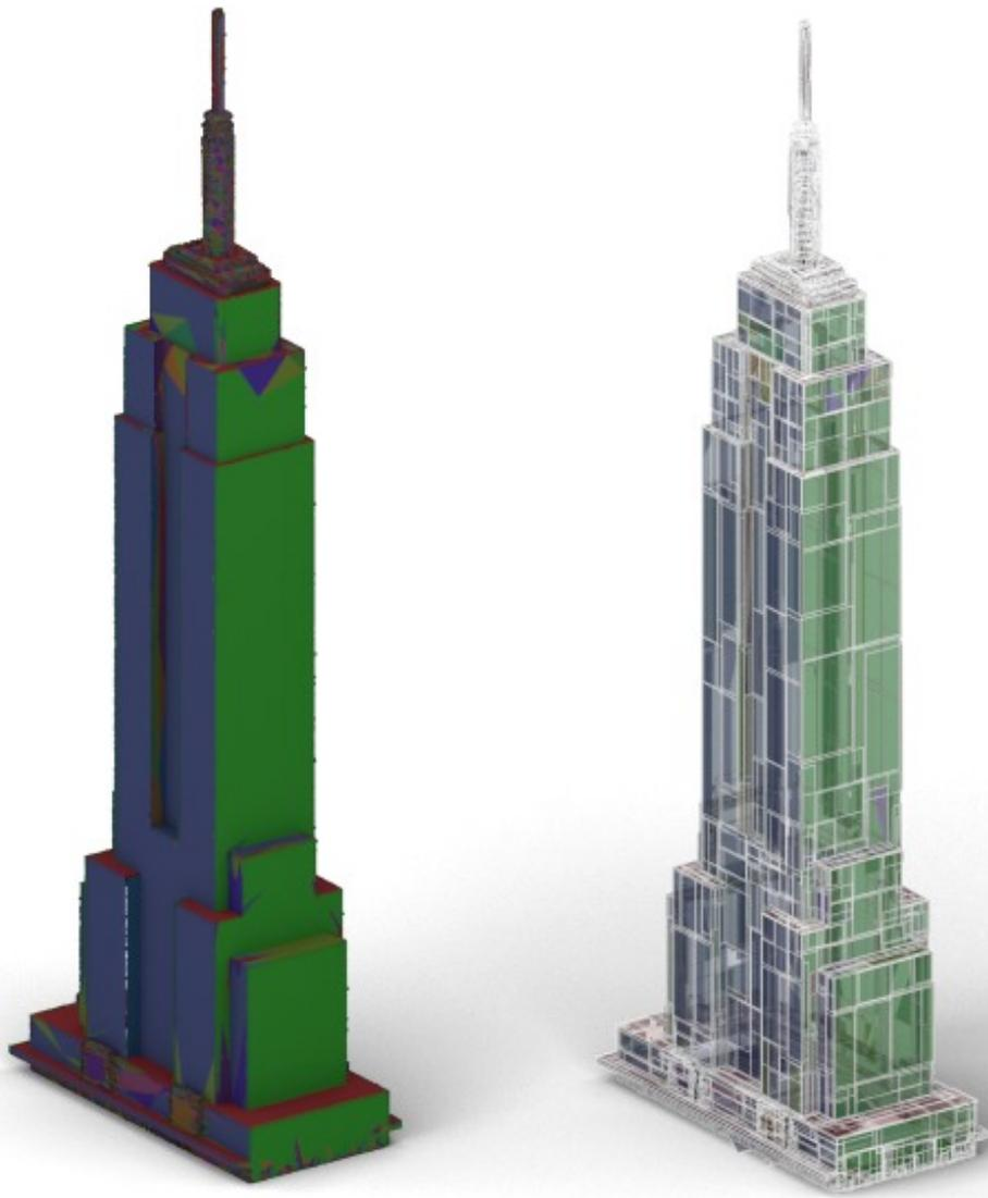
**Figure 19:** *Empire* (Figure 10), [Lafarge and Alliez 2013]: Reprojected cloud (left), planar polygons (right)
